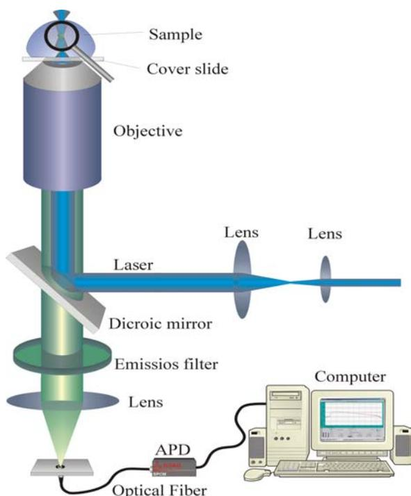
**Figure 2: Schematical drawing of an FCS setup**
