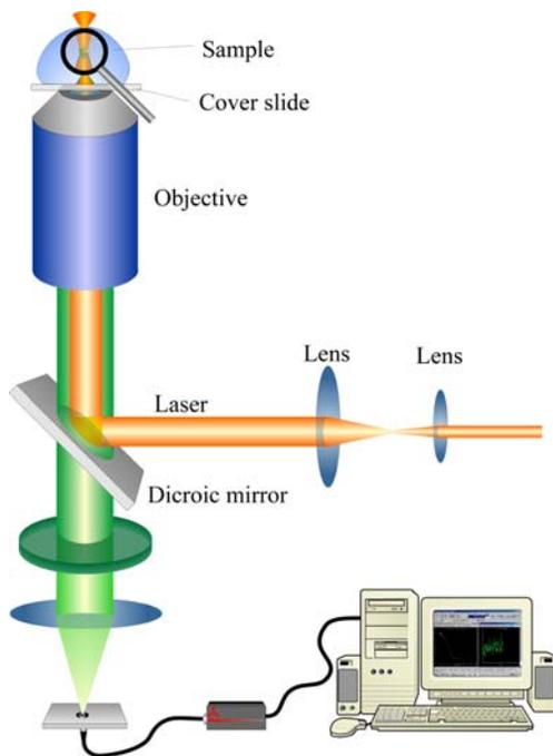
**Figure 6: Two-photon setup**
