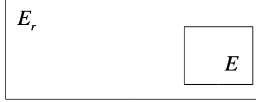
Figure 2.1: A system with energy E thermally coupled to a large heat reservoir with energy E_r .
