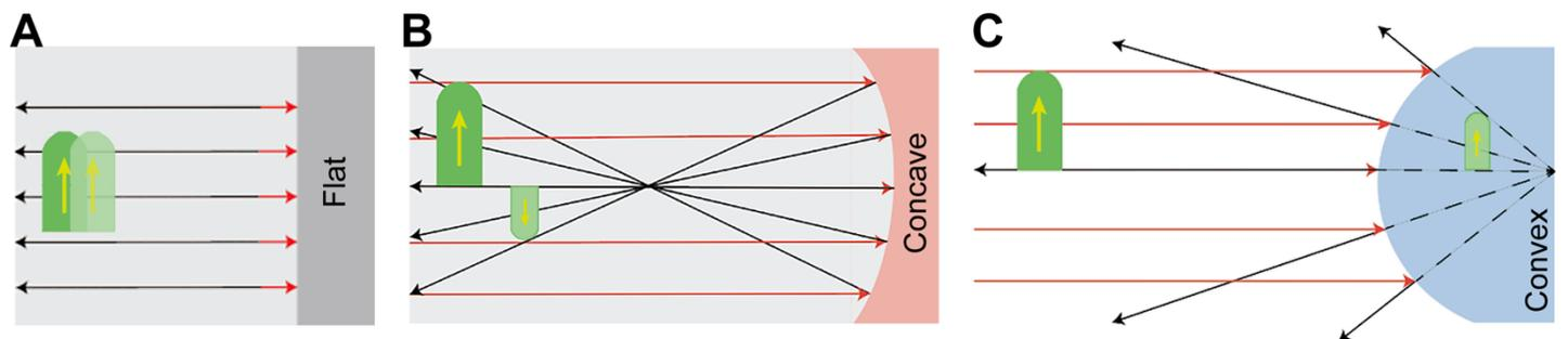
**Fig. 4** Images formed by flat and curved surfaces differ due to reflected light. **A**) Flat surfaces reflect light from the object (green) that forms a same-sized upright image of the object (pale green). **B**) Concave surfaces reflect light from the object that forms a small inverted image of the object. **C**) Convex surfaces reflect light from the object that forms a small upright image of the object.
