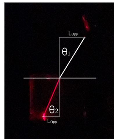
**Fig. 5** For Experiment 2, the index of refraction for water,  $n_2$ , can be calculated from the angle of light incidence (top,  $\theta_1$ ) and the angle of refraction (bottom,  $\theta_2$ ).
