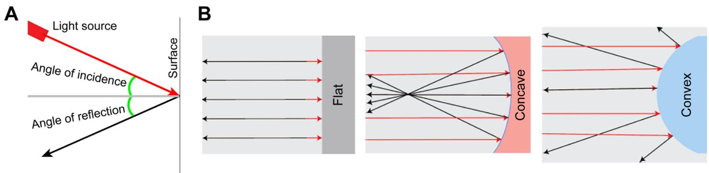
**Fig. 3** Reflection of light. **A**) Light is reflected from a surface at the same angle as it strikes the surface. **B**) Light rays (red lines) are reflected (black lines) at the same angle for each point of a flat surface (Left), but the angles differ for each point of curved surfaces (Middle, Right). Note that for each point on either a flat or curved surface, the angle of incidence is the same as the angle of reflection.
