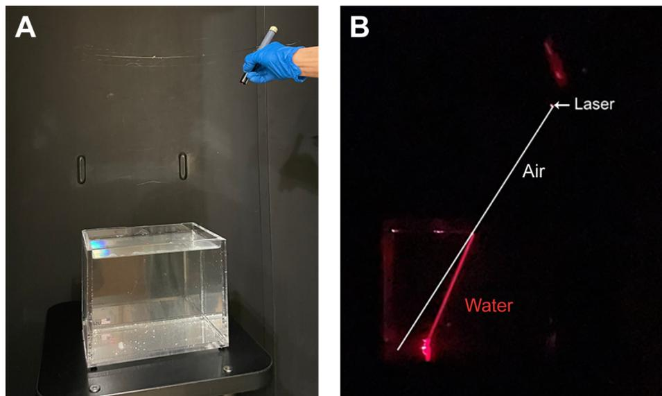
**Fig. 2 A)** Hold the laser pointer above the container of water so the laser light hits the water at an angle. **B)** Laser light in the dark. The laser light starts in air (top Right, arrow) and is visible in water as a red line (bottom). Laser light path in air (white line) and water (red line).
